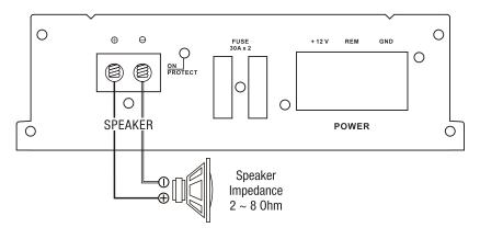
Please note that this units are mono block units and have only one channel. Connecting to either the positive or negative of either of the two connections will end in the same result as both positive connections (or both negative connections) are tied together inside the unit. For example, if you connect two 4 ohm subwoofers, the amp will parallel the connections for a 2 ohm load.
