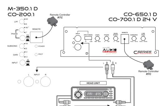
The M/C SERIES amplifier offers RCA-Inputs, which are connected through cinch cables with the preamplifier-outputs of the head unit. If the head unit (OEM-RADIO) has no RCA-Output, than it is possible to connect the speaker output direct to RCA/Cinch-Input of the amplifier.
